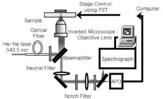
1. Schematic diagram of laser scanning microscope for single molecule and single cell detection.
